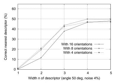
Figure 8: This graph shows the percent of keypoints giving the correct match to a database of 40,000 keypoints as a function of width of the  $n \times n$  keypoint descriptor and the number of orientations in each histogram. The graph is computed for images with affine viewpoint change of 50 degrees and addition of 4% noise.
