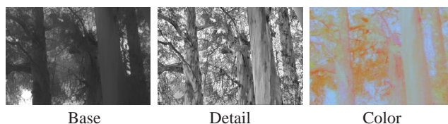
Figure 2: Principle of our two-scale decomposition of the input intensity. Color is treated separately using simple ratios. Only the base scale has its contrast reduced.
