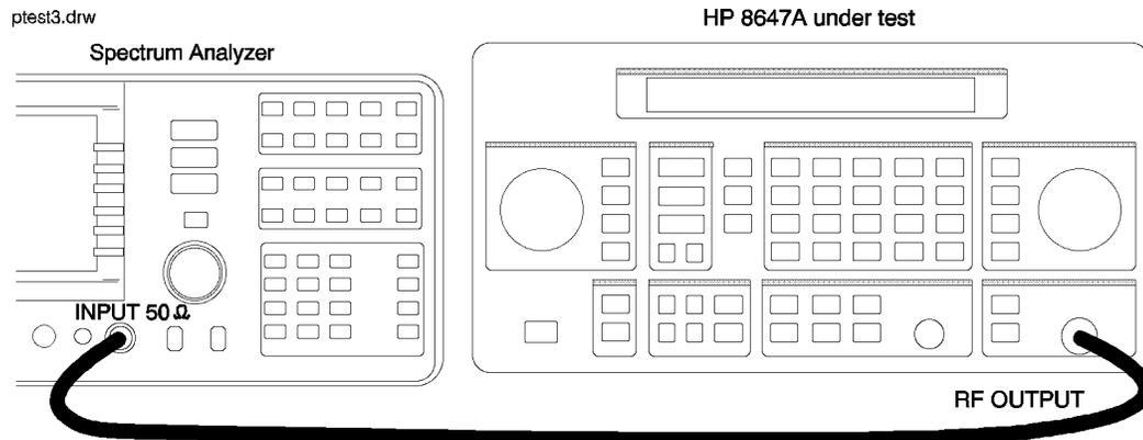
**Figure 8-9. Spurious Equipment Setup**
