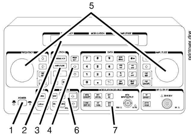
**1. Power Key** Press **POWER** to power-up the instrument. The instrument powers up to the same state it was in when power was turned off, except that the RF output will be turned off; press the **RF ON/OFF** key to turn it on.
