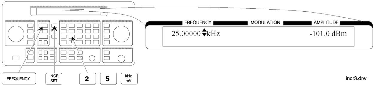
4. Increment the RF output frequency in 25 kHz steps.
