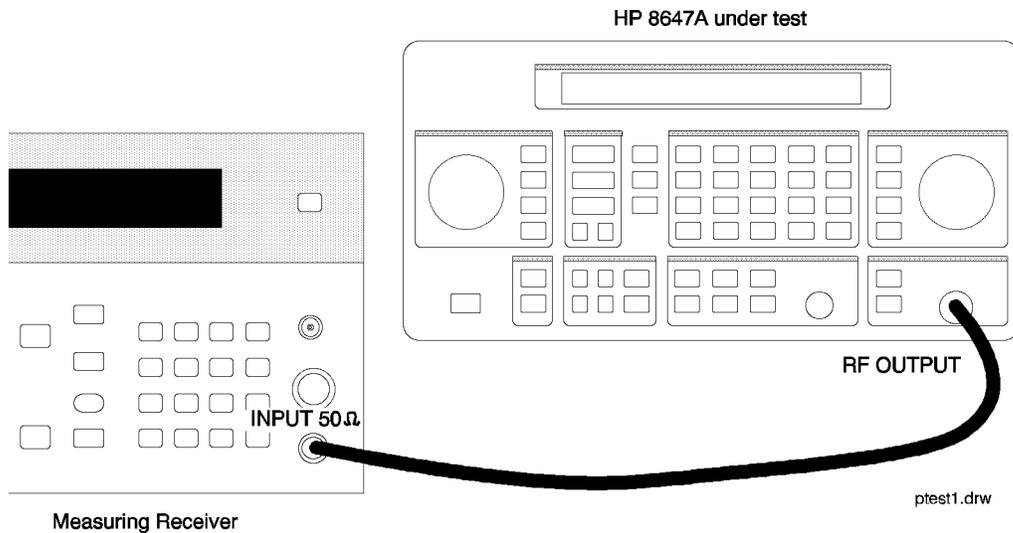
Figure 8-10. DC FM Frequency Error Equipment Setup
