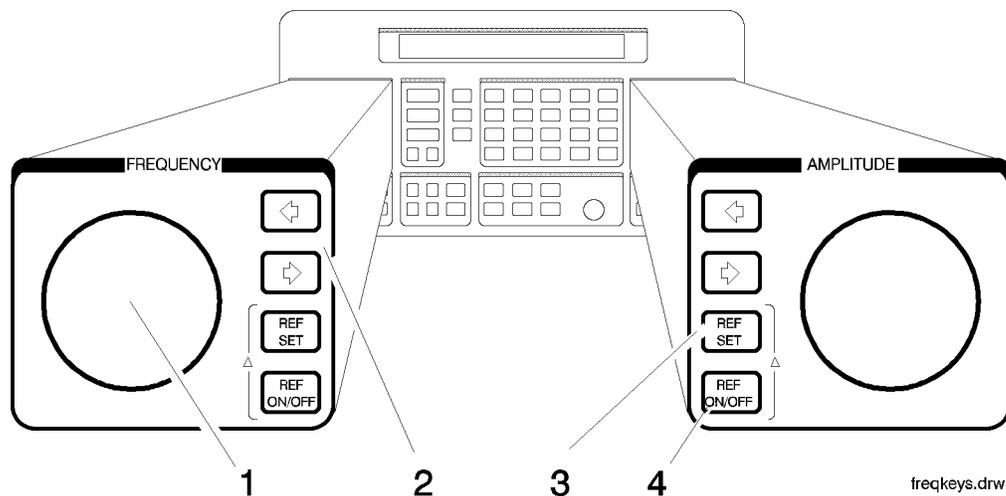
The knob and reference set keys work similarly for both frequency and amplitude.
