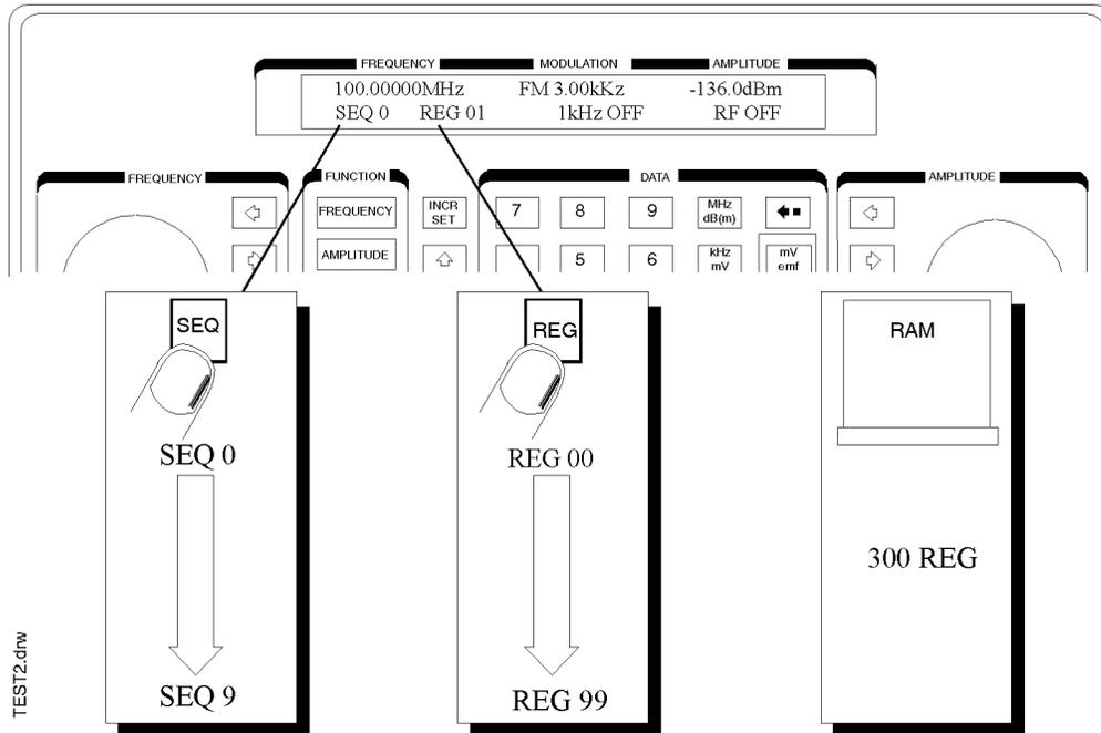
MEMORY key entries are automatically terminated after you enter the last digit. Register key entries ( **SAV**, **DEL**, and **REG** ), require two digits. Sequence key entries ( **SEQ** ) require one digit.
