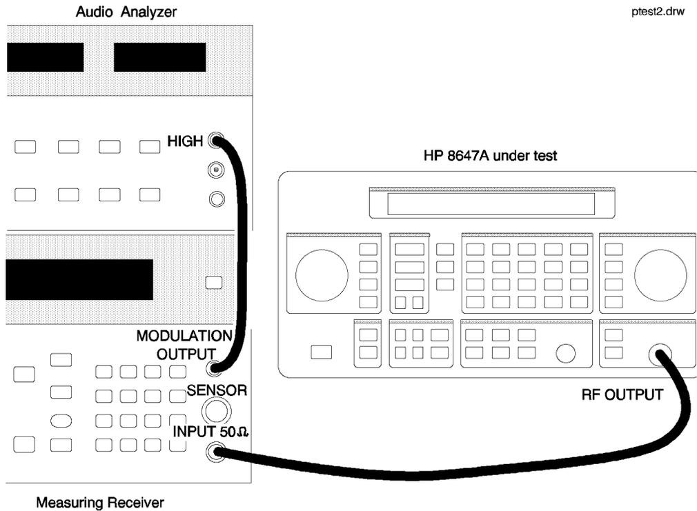
Figure 8-4. AM Distortion Equipment Setup
